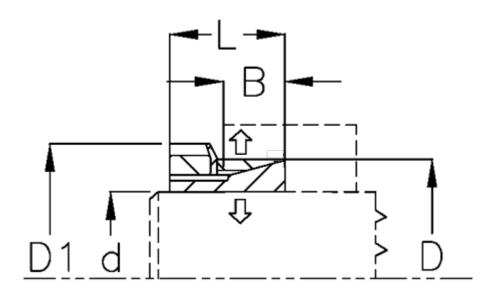
$\begin{array}{lll} \text{B mm} & = 8.0 \\ \text{D1 mm} & = 52 \\ \text{d H8 mm} & = 30 \\ \text{D mm} & = 40 \\ \text{Fit tolerance} & = \text{Aksel h8, Nav H8} \\ \text{F kN torque} & = 14 \\ \text{L mm} & = 20.0 \\ \text{P N/mm2 surface pressure on shaft/hub} = 80 \end{array}$
